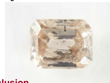
Fig. 6 Pink CVD diamond after LPHT annealing.
